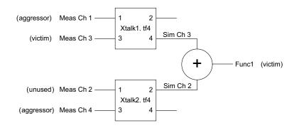
First, create two 4-port TFs (transfer functions) from two 4-port S-parameter models. Then, apply the two 4-port TFs to three measured signals in order to produce two simulated waveforms that can be added together using a waveform math function.
