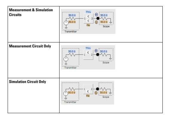
These choices let you build/view the measurement circuit, the simulation circuit, or both at the same time.
