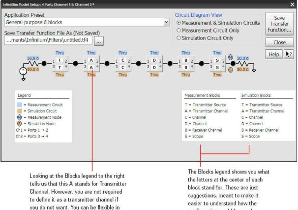
You can also change the name of a block by clicking on it and using the Block Name control in the subsequent dialog box.
