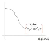
Notice that above a certain frequency (or bandwidth) there is very little signal and mostly noise. If you apply a correction through InfiniiSim as discussed above, you may end up excessively amplifying the noise. The **Bandwidth Limit** field in this dialog box lets you minimize this noise gain by attenuating the resulting waveforms above the frequency where there is mostly just noise.
