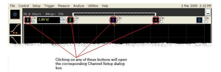
**2** After opening the Channel Setup dialog box, set the entry controls for your specific setup. You can see the InfiniiSim entry controls in the screen shot below.
