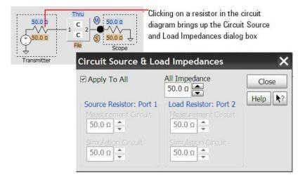
The Circuit Source and Load Impedances dialog box lets you specify all of the source and load impedances within both the measurement and simulation circuits.
