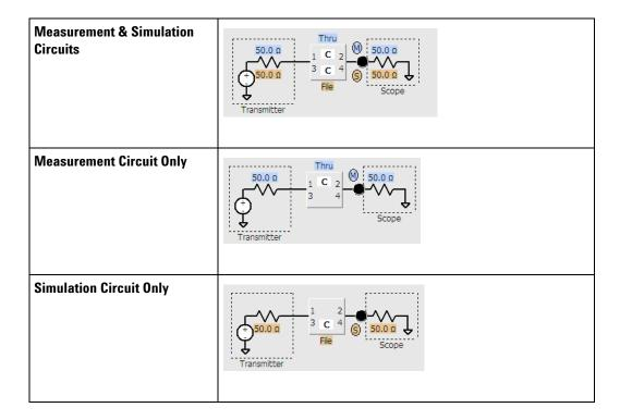
These choices let you build/view the measurement circuit, the simulation circuit, or both at the same time.
