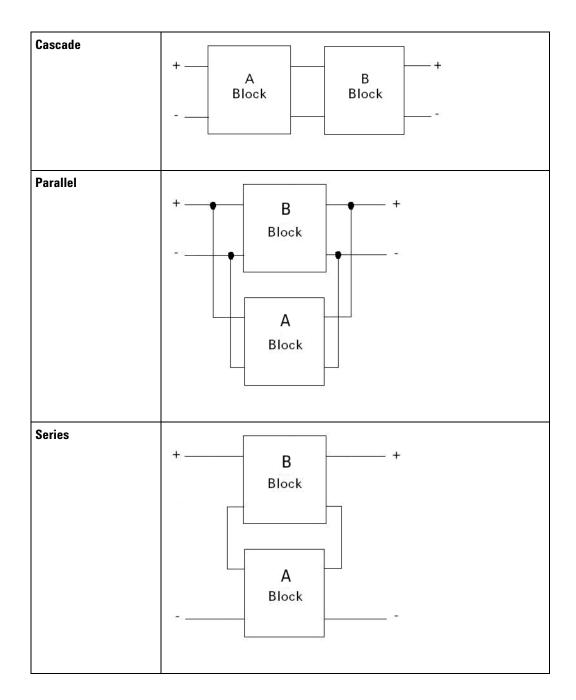
In **4 Port** port type mode, the 4 port blocks combine as shown below (pictures show connections for two of the three blocks for simplicity):
