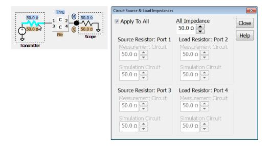
The Circuit Source and Load Impedances dialog box lets you specify all of the source and load impedances within both the measurement and simulation circuits.
