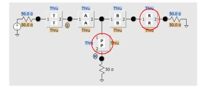
A probe must be connected to the channel in order for the **Probe** block type selection to be active.
