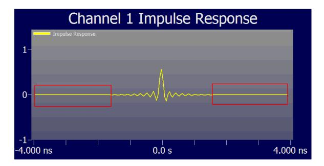
As you can see, there are large sections of the impulse response that are just flat and, therefore, contribute insignificantly to the simulated waveform. If you see this, you may be able to increase your measurement update rate by reducing the **Max Time Span** control.
