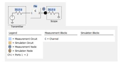
To get it set up like this, click the **C** block to open the InfiniiSim Block dialog box. Then, select the **Measurement Circuit** option in the Circuit section. Under Block Type, choose **S-parameter File** and then click the **S-parameter File** field, navigate to where you saved the file on the oscilloscope, and click **Load**. Because the S-parameters represent a cable,  $S_{21} = S_{12}$ , checking the **Flip Model** option should have no effect.
