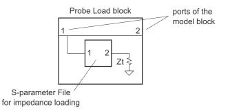
When you make the **Probe Load** block type selection, additional controls appear at the bottom of the dialog box:
