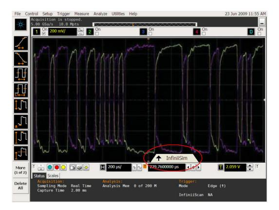
Click this tab to see plots of the frequency response of the original measured signal, the simulated signal, and the filter applied by InfiniiSim. You can also see the impulse response and step response plots of the transfer function as well.
