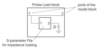
When you make the **Probe Load** block type selection, additional controls appear at the bottom of the dialog box:
