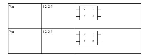
The **Port Extraction** field tells InfiniiSim how to extract a 2-port model from the 4-port S-parameter file and use it in your 2-port transformation.
