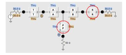
When the **Probe Load** block type is selected it does two things: port 1 and 2 of the block are connected together (like an Ideal Thru) and the supplied S-parameter file is used to describe the shunt impedance loading the connected ports.
