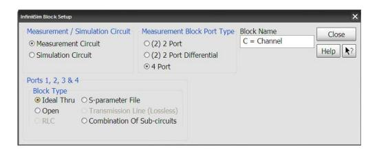
The first section (**Measurement/Simulation Circuit**), lets you specify whether you are currently defining a block in the measurement circuit or the simulation circuit. For instance, if you select **Simulation Circuit** in this section and then set the **Block Type** to **Ideal Thru**, then the corresponding block in the simulation circuit is set to a Thru block.
