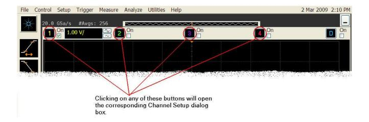
This opens the Channel Setup dialog box. Under the **InfiniiSim** section, select **2 Port** (we assume the signal passing through the cable is single-ended). Then, enable the **Bandwidth Limit** field and set it to to **4 GHz** because we assume our signal to noise ratio past 4 GHz is low (either we already know this or we determined it from the "Frequency Response Plot" on page 63). Click the **Setup...** button to open the InfiniiSim Setup dialog box.
