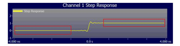
The screen shot above shows the large flat areas enclosed by red rectangles. You may need to reduce the **Max Time Span** control in this instance.
