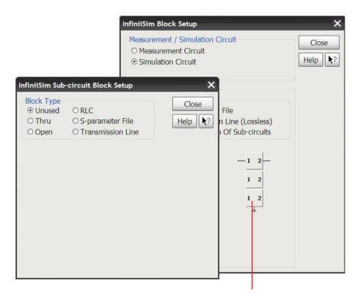
Clicking on one of these blocks will bring up its corresponding InfiniiSim Sub-circuit Block Setup dialog box where you can define it
